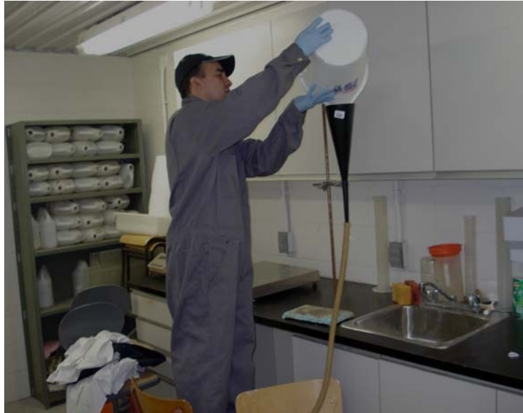
Fig 3.1: Experimental set-up to compare hog manure flow characteristics.
